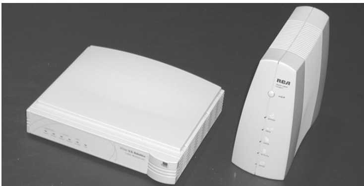
Figure C.4 Cable Modems for Cable Internet Access, Manufactured by 3Com (left) and RCA (right)
