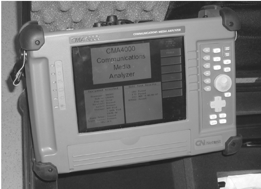
Figure 0.8 OTDR (Optical Time-Domain Reflectometer)
