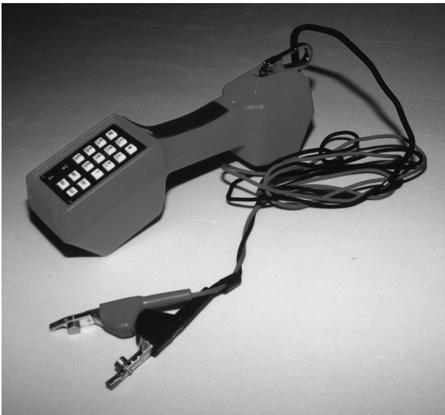
Figure C.36 Harris Dracon Craft Test Set (Also Known as a “Butt Set” or “Goat”).
