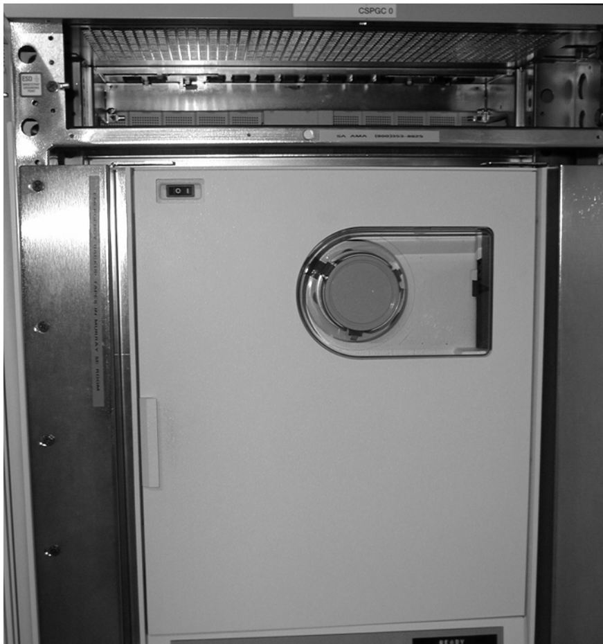
Figure M.2 A Magnetic Tape Back Up for a Lucent Technologies 5ESS Central Office Voice Switch
