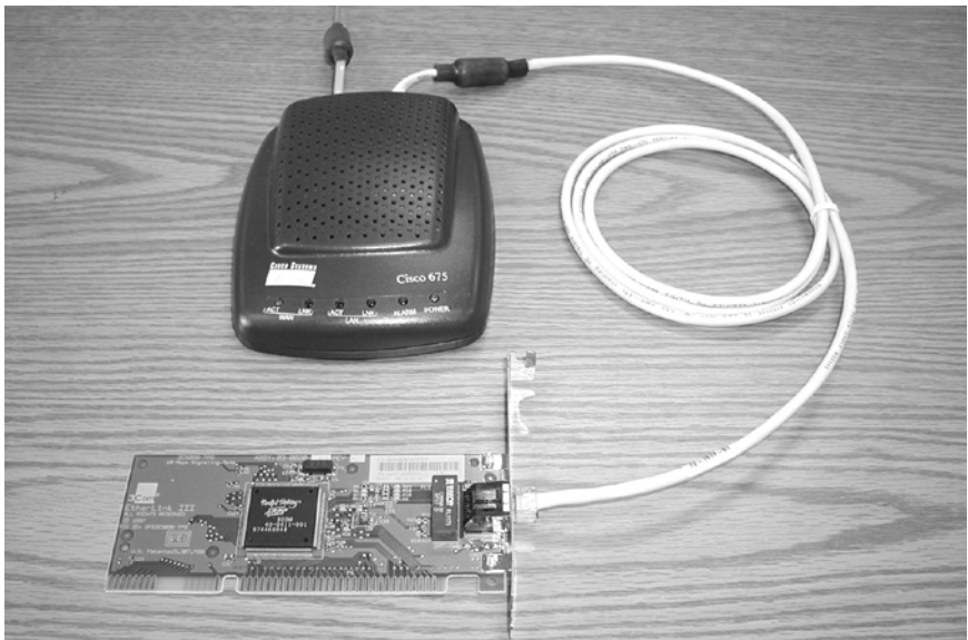
Figure A.7 ADSL Router
