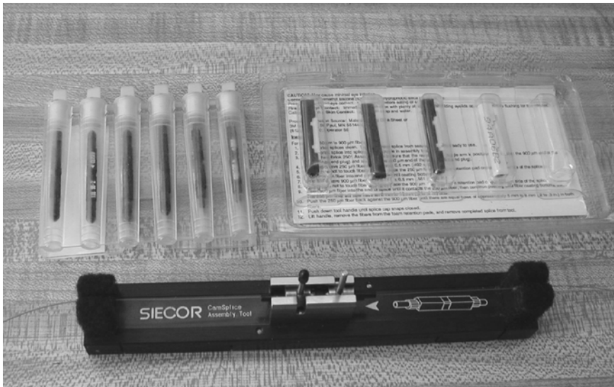
Figure M.6 Fiber-Optic Kit for Mechanical Splices
