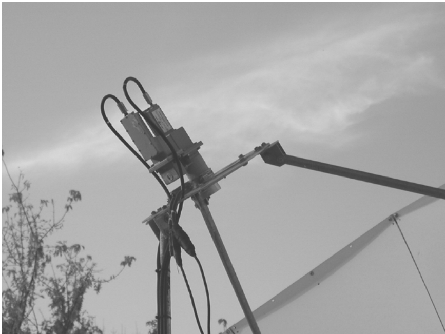
Figure F.3 A Feedhorn with LNB Converter Attached Above the Satellite Dish
