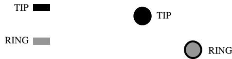
Figure T.16 Tip and Ring Positioning on Blocks and Terminals. Tip is on Top (Left) and Ring is on Bottom (Right)
