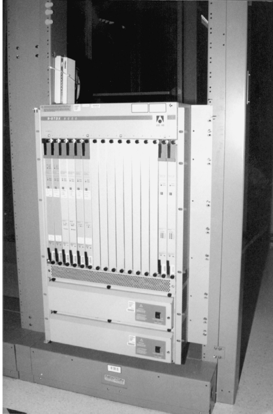
Figure F.16 Frame Relay Switch/Mfg. by Ascend
