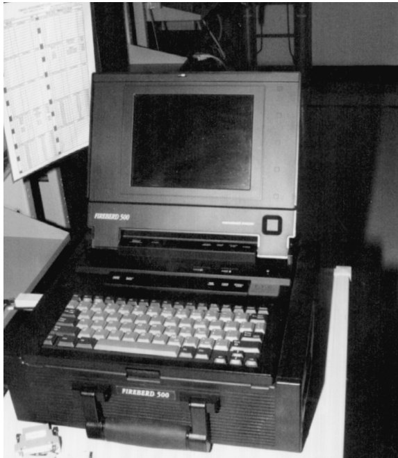
Figure P.29 A Firebird 500 Protocol Analyzer, Manufactured by TTC
