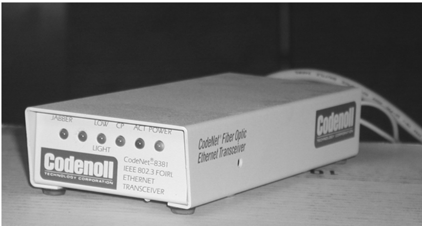
Figure T.18 Transceiver: Ethernet Category 5 UTP to Single-Mode Fiber Optic
