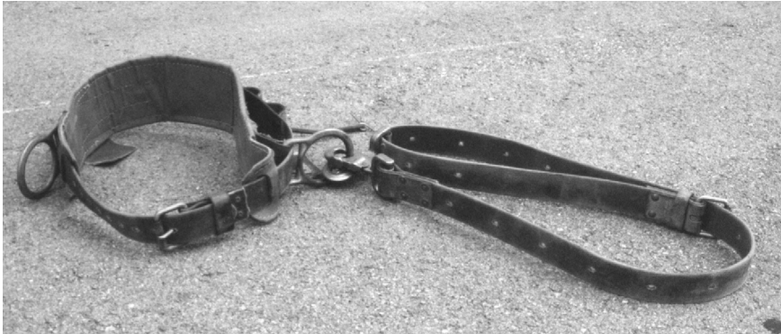
Figure S.1 A Safety Belt (Also Called a Body Belt or Climbing Belt ).
