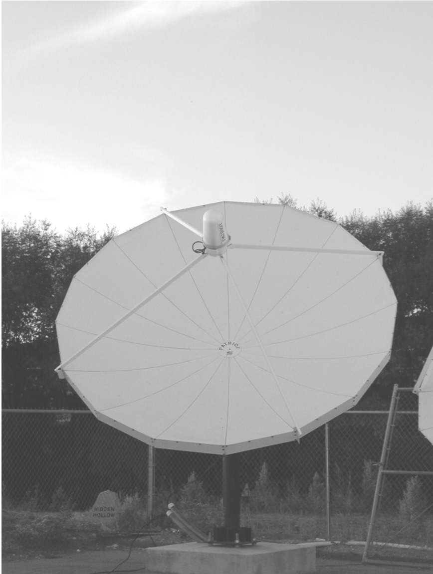
Figure P.3 Parabolic Dish Antenna: 3.7 Meter With C-Band LNB
